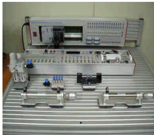
Figure 1. A conventional PLC training system (mostly used in South Korea)
